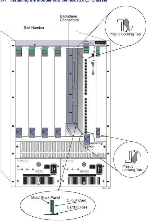
Figure 3-1 Installing the Module into the MATRIX E7 Chassis
